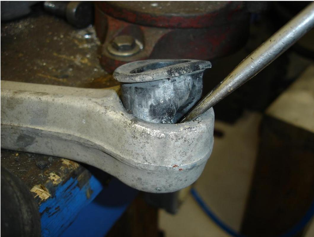
The rubber bushing is easily coaxed out of the rod end once the sleeve is removed. Kits that do not provide new sleeves will require you to clean up the old sleeve of any rubber remaining on the sleeve.
