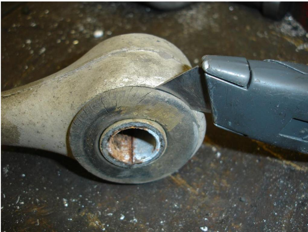
Using a razor knife to remove the outer lip of the rubber bushing allows it to push out easier. If you do not have a vise or press to push the bushings out, some opt to use a drill bit to cut through the rubber between the bushing and sleeve. Using the razor blade first will also give you an idea of what diameter drill bit to use, care must be taken that you do not drill into the control arms soft aluminum.
