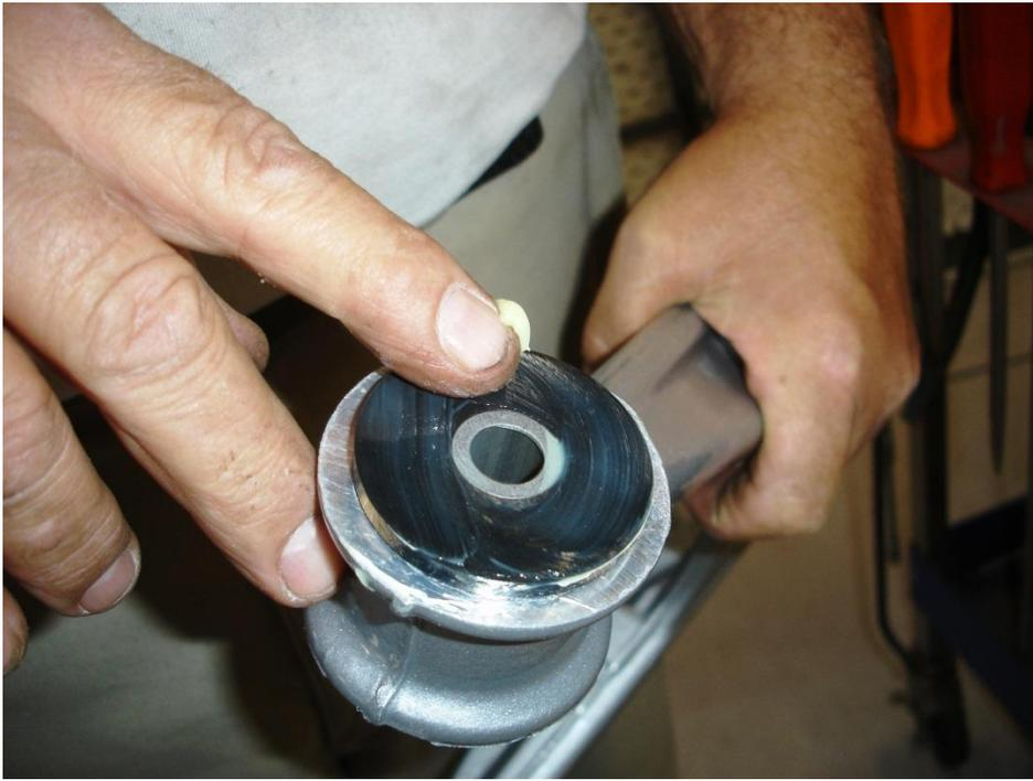
Before installing the control arm or rod end into the pivot point a coat of silicone will help alleviate squeaking as the bushing pivots. All suspension pivot bolts should be torqued to GM service manual specifications after assembly. Loose bolts cause clunking and or popping noises as you go over bumps.
