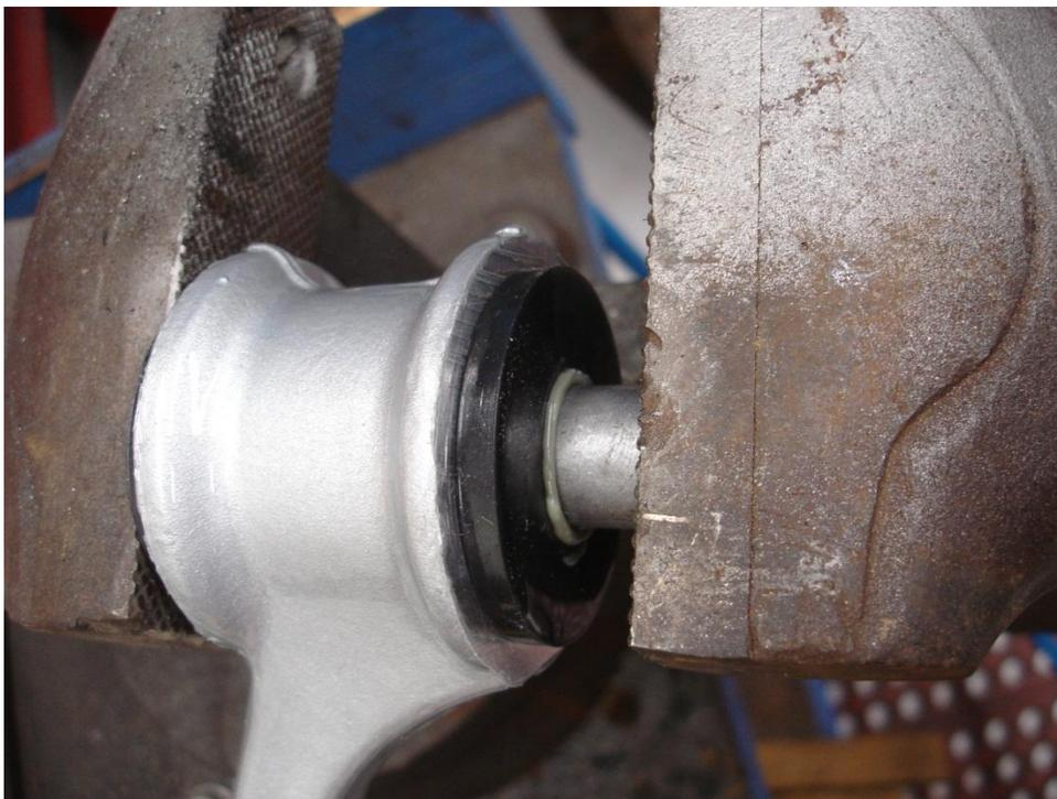
Silicone grease should be applied to the outside of the sleeve and some should also be applied to the bushings inner surface. The sleeve should rotate on the bushings inner surface, here a bench mounted vise is used to push the sleeve into the bushing halves.
