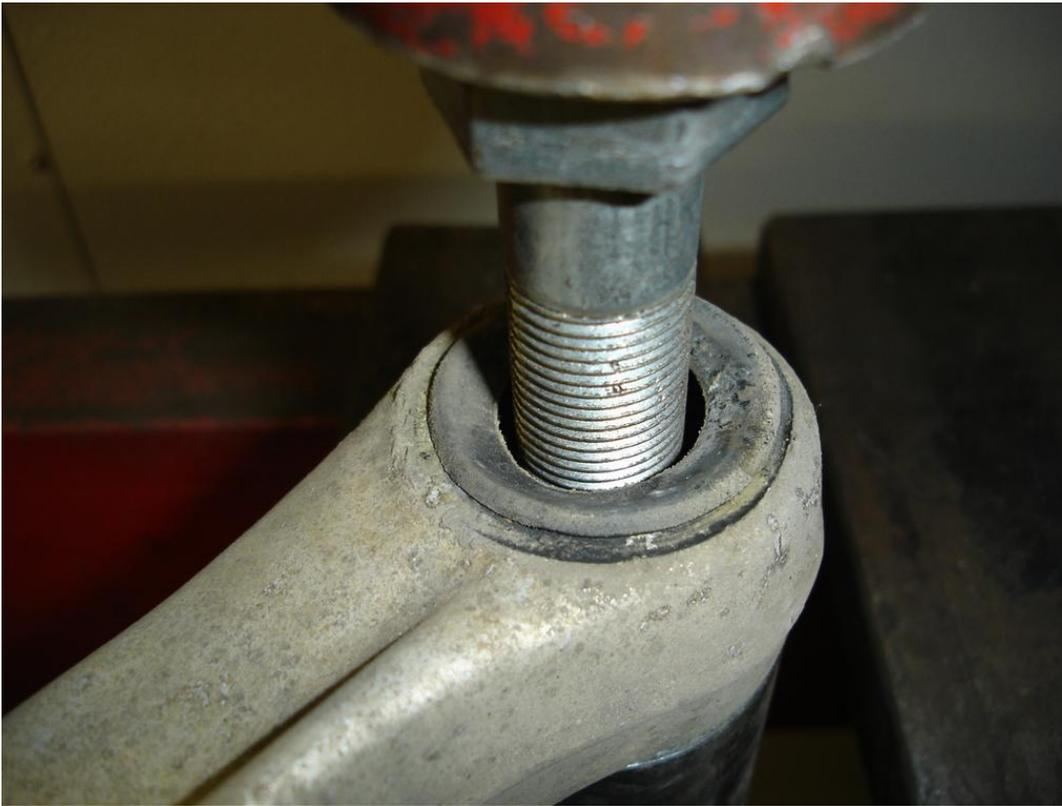
Very important to remember the bolt we are using is smaller diameter than the sleeve to keep from sticking the push bolt in the rubber. All sleeved bushings can be handled in this manner C2 through C6 Corvettes.
