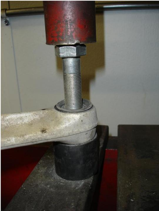
This is the easy way, using a sleeve larger than the rubber bushing to receive the bushing as it is pushed out. The hydraulic press does the hard work forcing the rubber bushing out. A vise can also be used in this manner but it takes more effort to get things moving.
